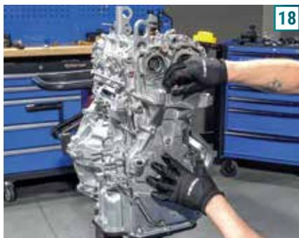
**19)** Instale as válvulas VVT, aplicando o torque de 10 Nm.
