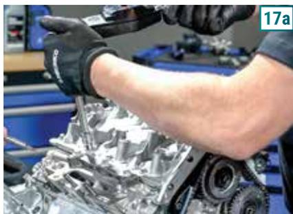
**17)** Instale as tampas do cabeçote, aplicando o torque de 10 Nm.
